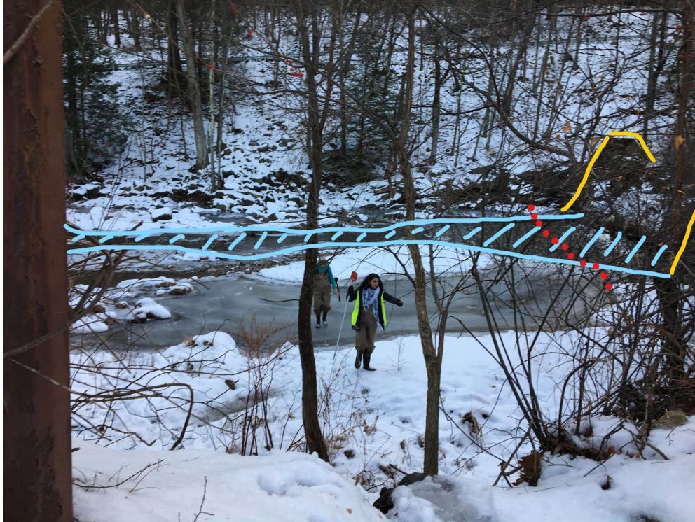
Figure 7-15: Flowing Water Shown in Blue; Dam Abutments Shown in Orange; Path of Data Collection Shown in Red
