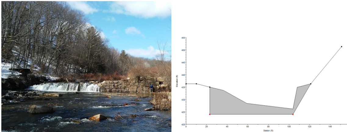
Figure 11. Photo of Brassworks Dam (Left) and HEC-RAS Screenshot Showing the Brassworks Dam Modeled as an Inline Structure (Right)
