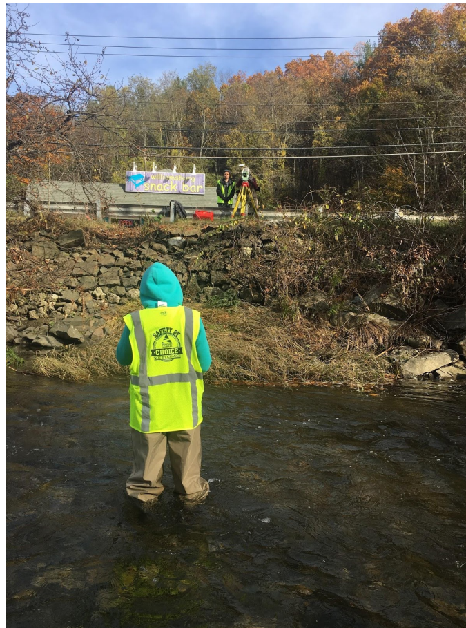
Figure 7-12: Collecting data, facing total station with receiver (Fereshta) in the river
