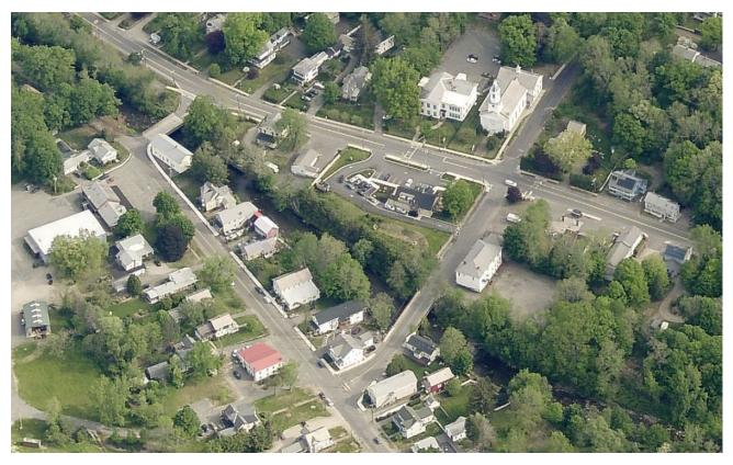
This bird's-eye view of Haydenville shows the close relationship between the village center and the river. The Bridge Street and South Main Street bridges shown are at risk of scouring and occasional overtopping during severe storms. A current MassDOT project is redesigning the bridges.
