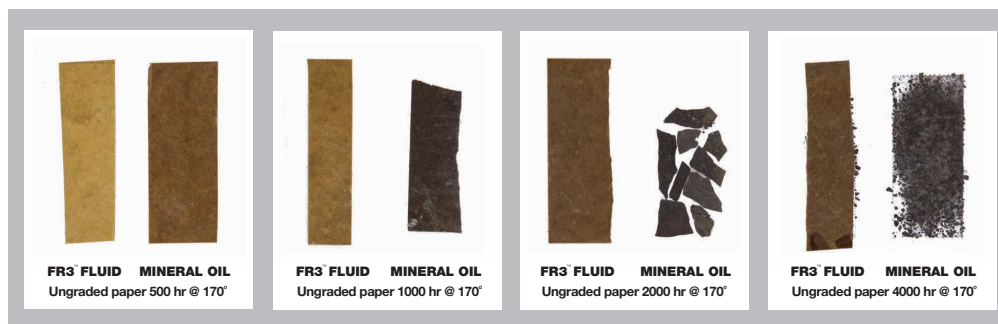
Insulation aging study comparing thermally upgraded paper using FR3 fluid vs. mineral oil.
