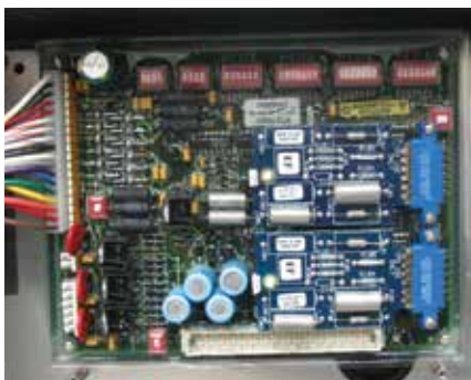
Figure 8. Typical Tri-Phase Control TCC module.
