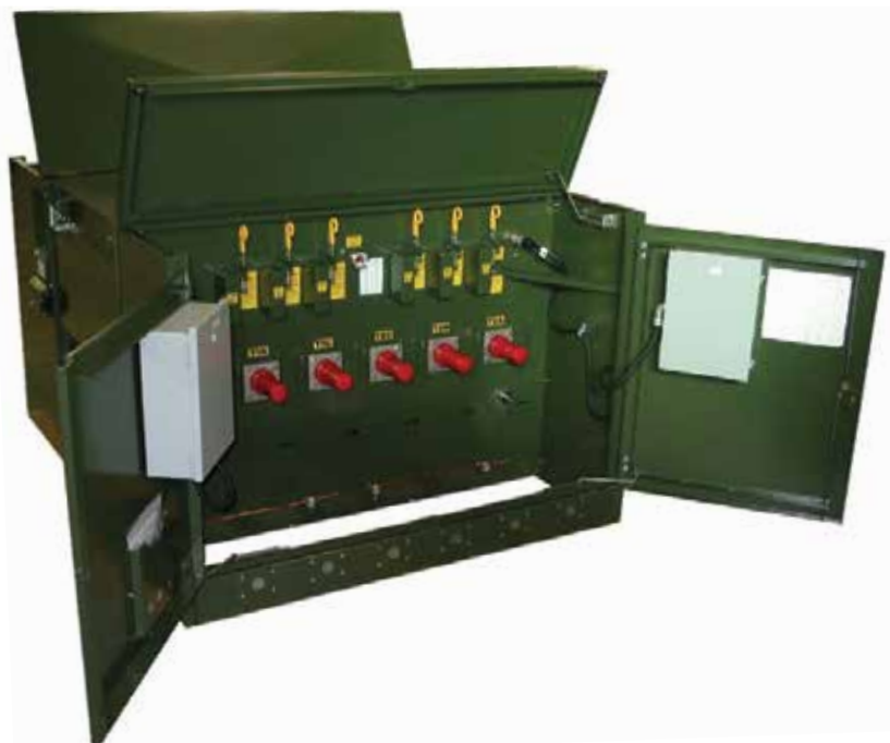
Figure 1. VFI underground distribution switchgear offers a simplified approach to the protection of 15, 25, and 35 kV underground systems, and provides a wide choice of switching combinations to meet system requirements.
