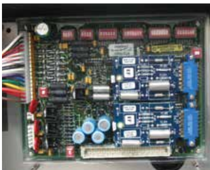
Figure 8. Typical Tri-Phase Control TCC module.
