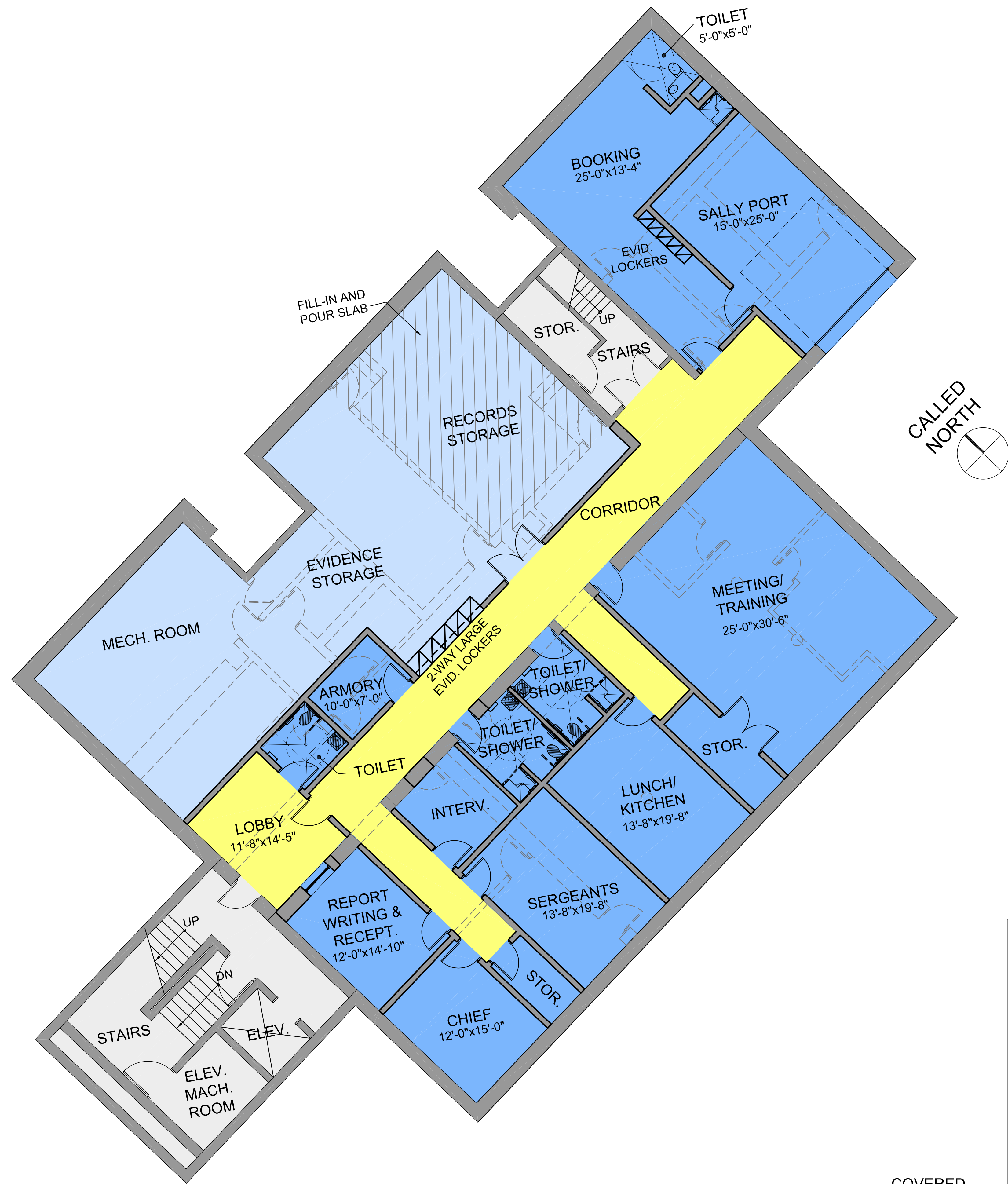
1 POLICE DEPARTMENT FLOOR PLAN 1/8" = 1'-0" NET FINISHED AREA: 4,286 S.F. NET SEMI-FINISHED AREA: 2,446 S.F. OVERALL GROSS AREA: 7,480 S.F. (BASED ON STUDY BY COLLIERS INTERNATIONAL)
